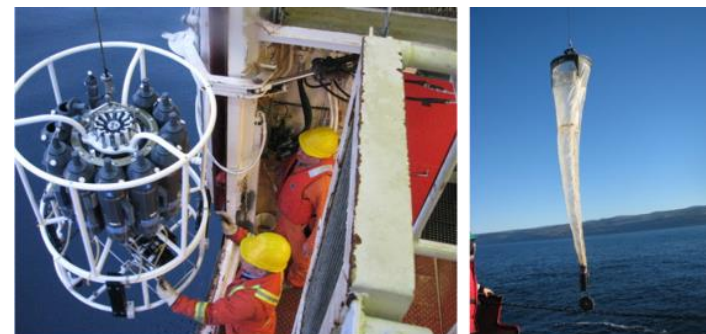
Figure 1: Sampling of water using a rosette and sampling of zooplankton using a vertical net.
